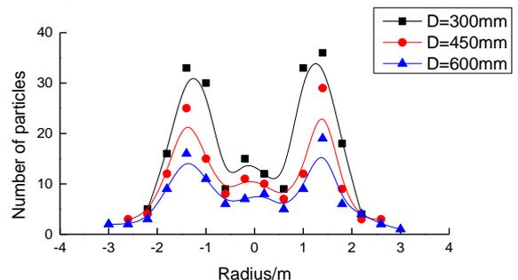
Figure 7. variation of number of particles with distribution radius in each selected rectangular region with different diameter of the distributor
