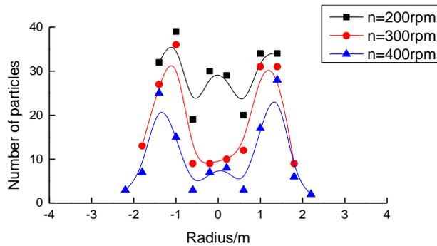
Figure 8. variation of number of particles with distribution radius in each selected rectangular region at different rotation speed of the distributor
