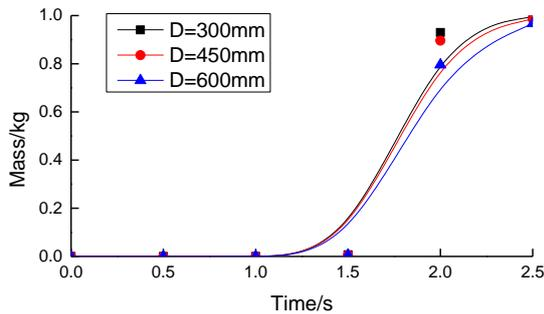
Figure 4. variation of mass with time in the selected region with different diameter of the distributor
