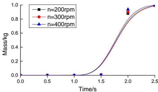
Figure 5. variation of mass with time in the selected region at different rotation speed of the distributor.
