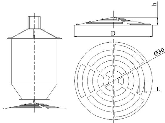
Figure 1. The structure view of the distributor
