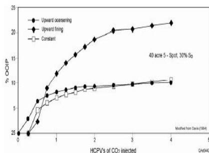
Figure 13. Upward-finishing sedimentation displaying best recovery character, reaching over 20% of OOIP.
