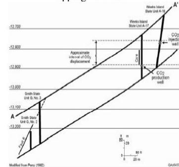
Figure 8. Weeks Island pilot with oil production at the base of the sandstone and approximately 100 ft of vertical displacement.
