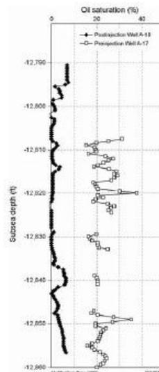
Figure 3. Residual oil saturation varying through a vertical sandstone profile.
