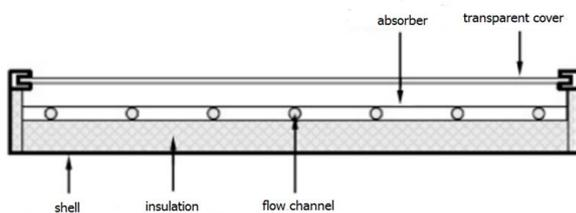
Figure 1. The structure of flat plate solar collector
