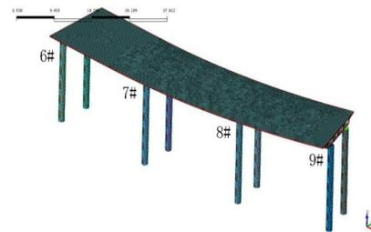
Figure 1. Structure finite element model
