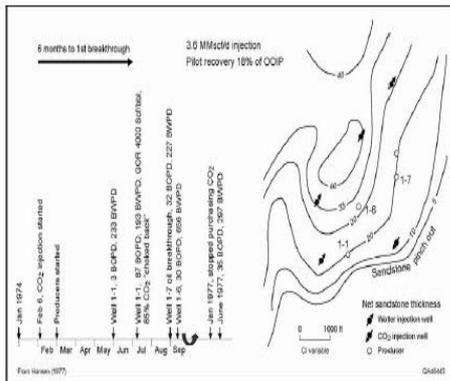
Figure 10. Little Creek field pilot consisting of one injector, four producers, and a curtain of four water injectors.
