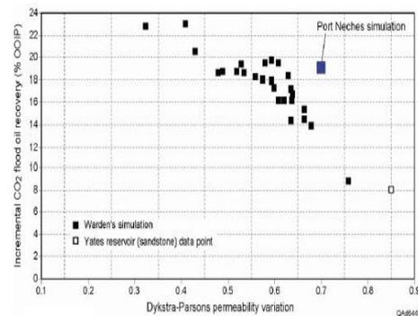
Figure 12. Increasing vertical permeability variation decreasing CO<sub>2</sub> EOR recovery efficiency.
