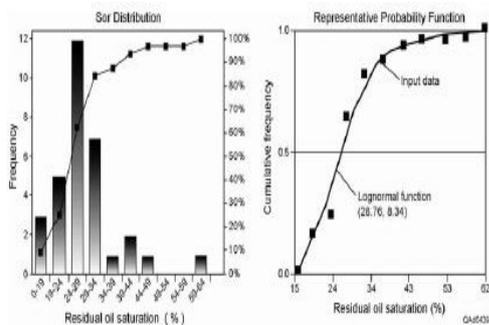
Figure 2. Distribution of average reservoir residual oil saturation in Frio fluvial-deltaic reservoirs ranging from 0.1 to 0.6, with a median of 0.26.
