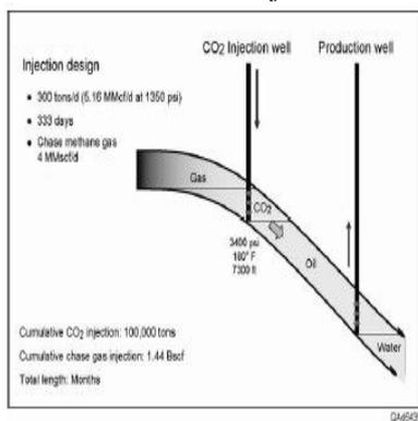
Figure 6. In Timbalier Bay gravity-stable flood CO<sub>2</sub> injected right below the gas cap.
