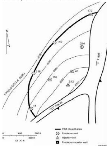
Figure 5. Injector at the top of the structure in water-after-gas (WAG) flood for the Quarantine Bay pilot.
