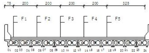
FIGURE 4 Static load test measuring point layout
