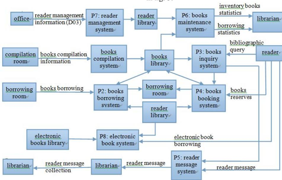
Figure 3. Functional module structure of library computer management system.
