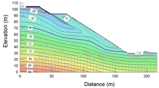
Figure 10. Simulation transient step1 pressure head contours
