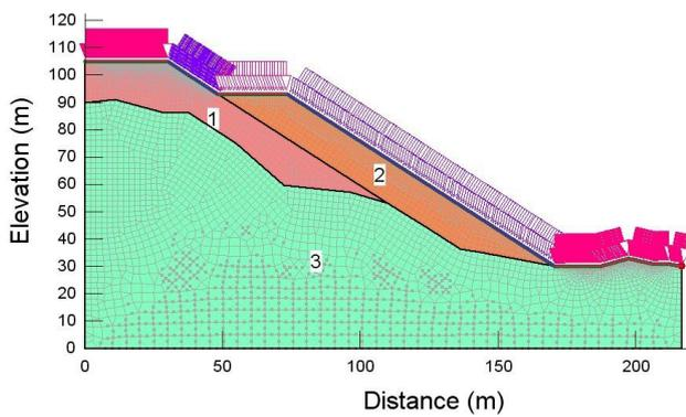
Figure 7. Simplified calculation model of the seepage finite element
