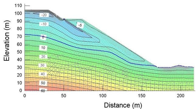
Figure 13. Simulation transient step2 pressure head contours
