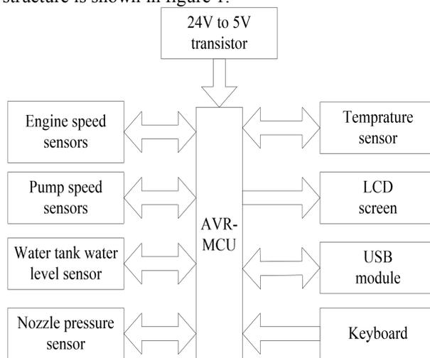
Figure1. Hardware structure
