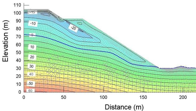
Figure 16. Simulation transient step3 pressure head contours
