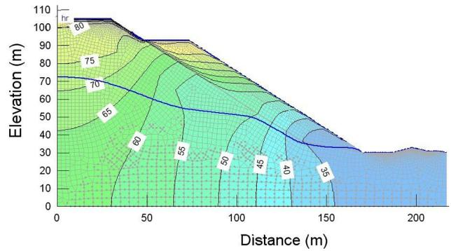
Figure 11. Simulation transient step1 total head contours
