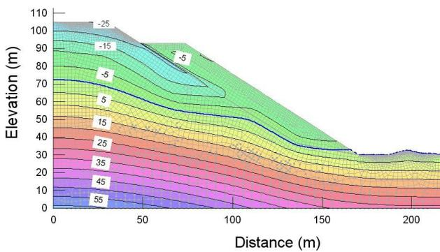
Figure 8. Simulation steady state pressure head contours
