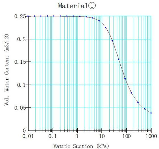
Figure 5. Water and soil characteristic curve
