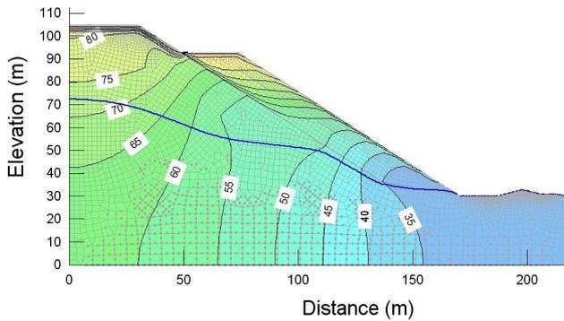
Figure 14. Simulation transient step2 total head contours
