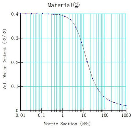
Figure 6. Water and soil characteristic curve
