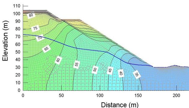
Figure 17. Simulation transient step3 total head contours
