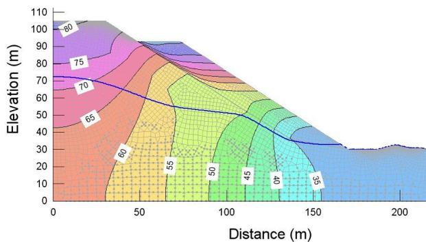
Figure 9. Simulation steady state total head contours
